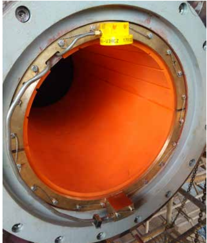
COMPAC propeller shaft bearing with Bearing Condition Monitor (BCM) System
