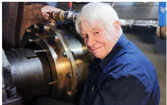
Sandy Thomson, onboard the Canadian Coast Guard Ship Hudson with SeaThigor Mechanical Face Seal installed.
